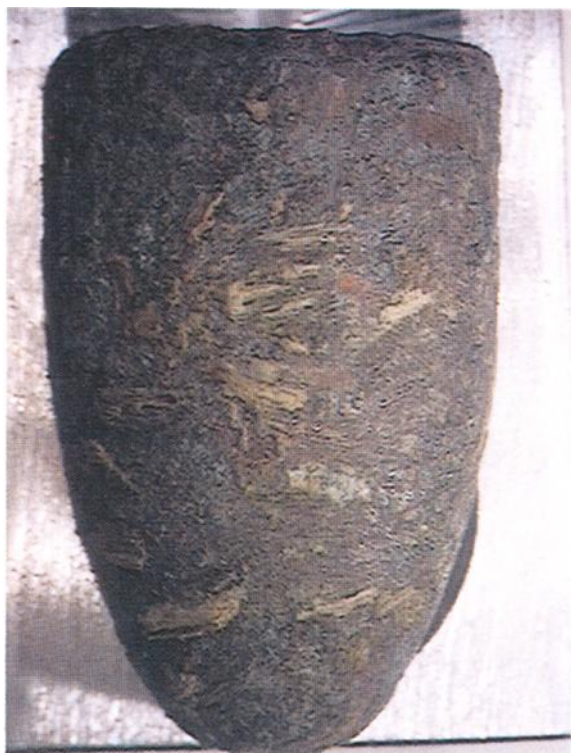
FIG. 3—Representative 9-mm bullet removed from the residence palm tree. Heavy corrosion and fragments of plant material strongly adhered to the surface (original magnification \sim 7\times ).
