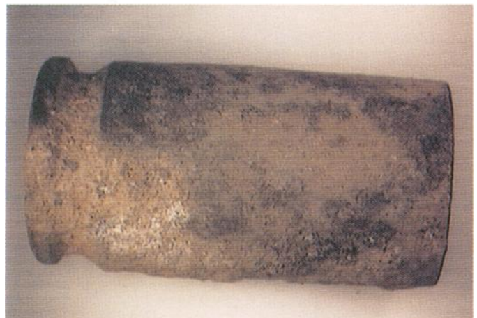
FIG. 2—Side view and end view of representative 9-mm casing recovered from the yard of the suspects' residence (original magnifications ~5× and ~8×, respectively).
